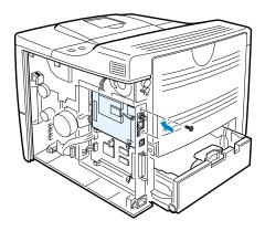
Replace the control board cover and tighten the two screws.
